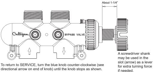
directional arrow on end of knob) until the knob stops as shown.
